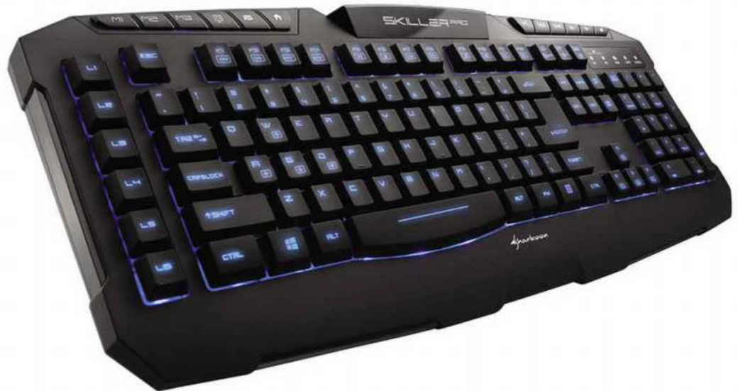
▲ The rubber dome membrane keys offer a near Cherry MX switch feel
